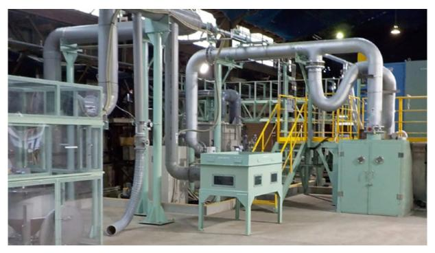
A new pilot plant operated by Sumitomo Metal Mining Co., Ltd., is testing a process for recovering and recycling cobalt from lithium ion batteries. Photo courtesy of Sumitomo Metal Mining
